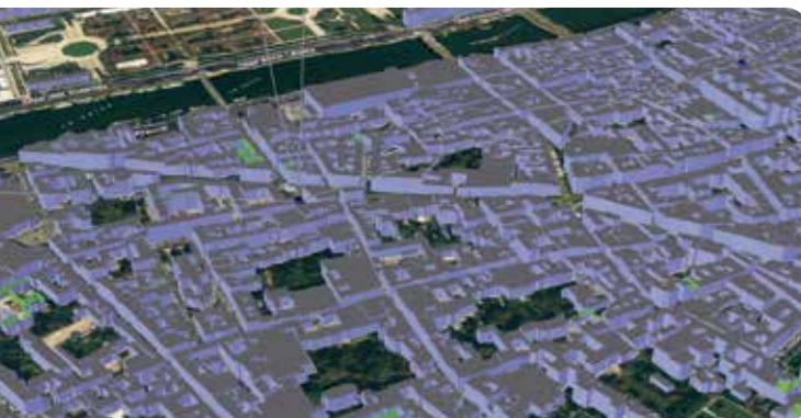
▼ 3D building layer for 5G network planning in a dense urban area.
