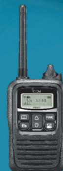
IP100H Terminal IP
